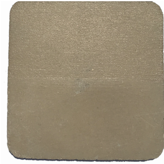
ADJACENT CONCRETE PAVING WITH DECORATIVE SCORE JOINTS APPLICATION: DECORATIVE PLAZA PAVING COLOR: DAVIS SANDSTONE
